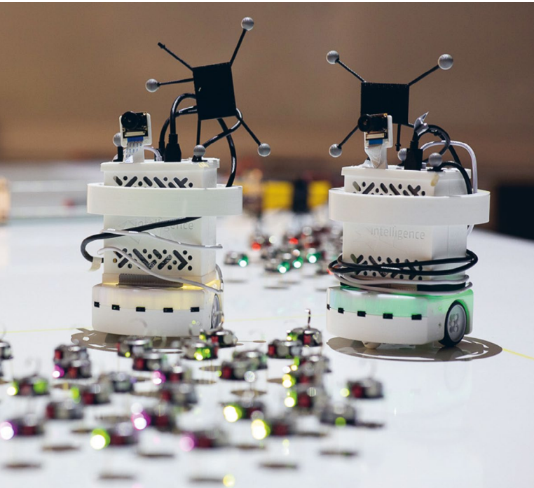
A group of Kilobots and, behind, two Thymios. These are SCIOI’s two fleets of swarm robots
